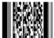
2D Code with stacked bar codes (stacked bar code type)
